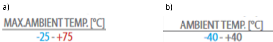
Fig. 2.5. Excerpts from the luminaire data sheets with the indicated operating temperature range [source: https://issuu.com/luglightfactory/docs/lug_into_led_07_2020_pl_web?fr=sYWUzMjE2MzMzODA ].
