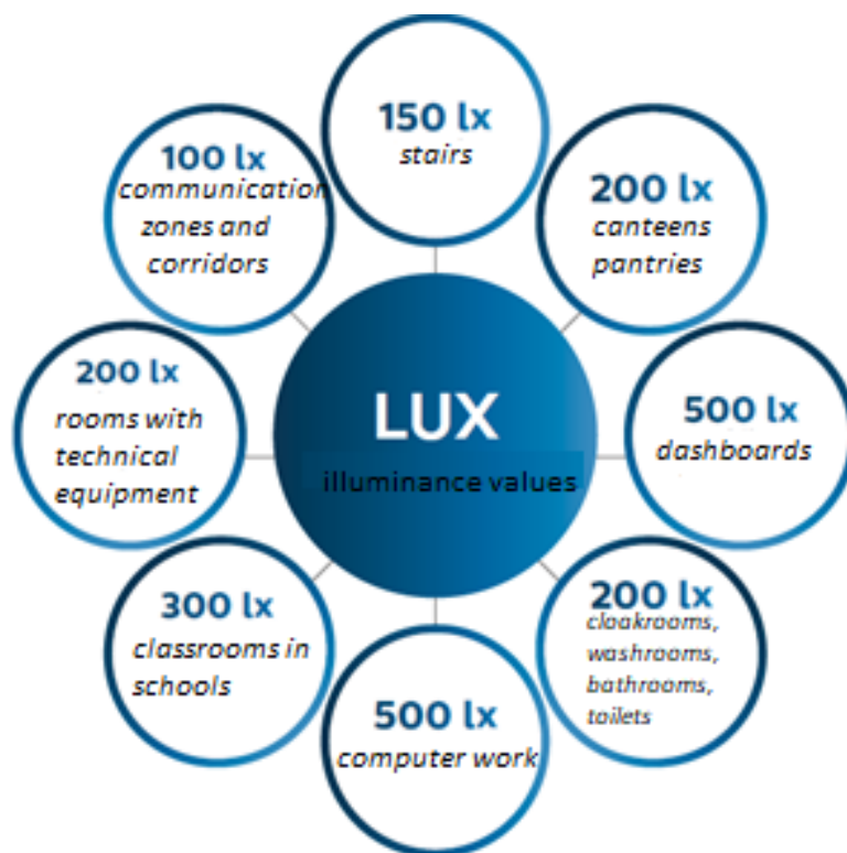
Fig. 2.6. Examples of selected illuminance values according to the standard EN-12464 [7], [source: https://www.elektroklub.pl/aktualnosci/news,162,jakie-miary-opisuja-swiatlo.html ].
